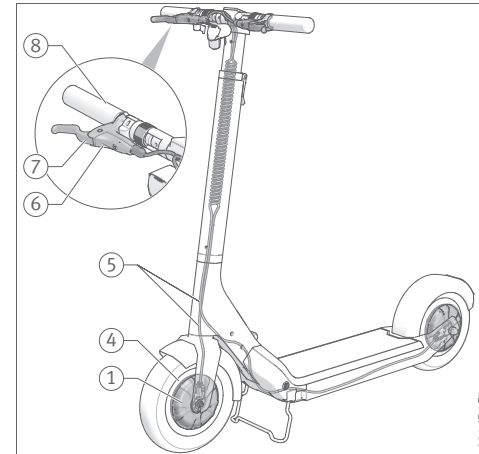
① Concentric brake cylinder, ④ Rim, ⑤ Brake lines, ⑥ Brake levers, ⑦ Lever blade, ⑧ Handlebars
